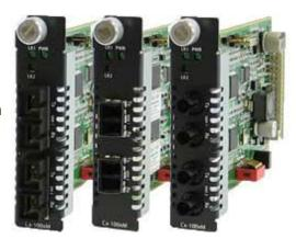
Installed in a high density Perle Media Converter Chassis, Perle's feature rich C-100MM Fast Ethernet Fiber to Fiber Media Converter Module enables transparent fiber extension of 100Base-FX multimode fiber to 100Base-FX multimode or 100Base-LX/EX/ZX/BX single mode fiber.
